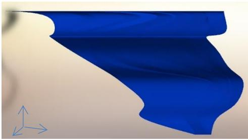
**Fig. 11.** 3D depiction of crack of sample 1
