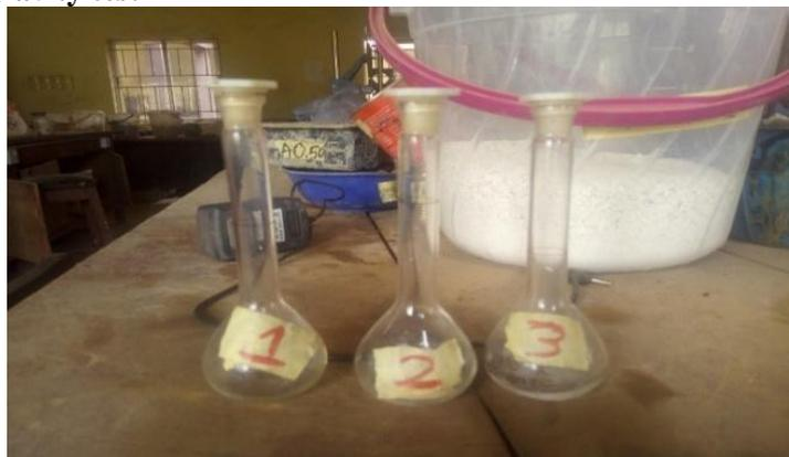
**Fig. 1.** Specific gravity test of bentonite and kaolin used in the study
