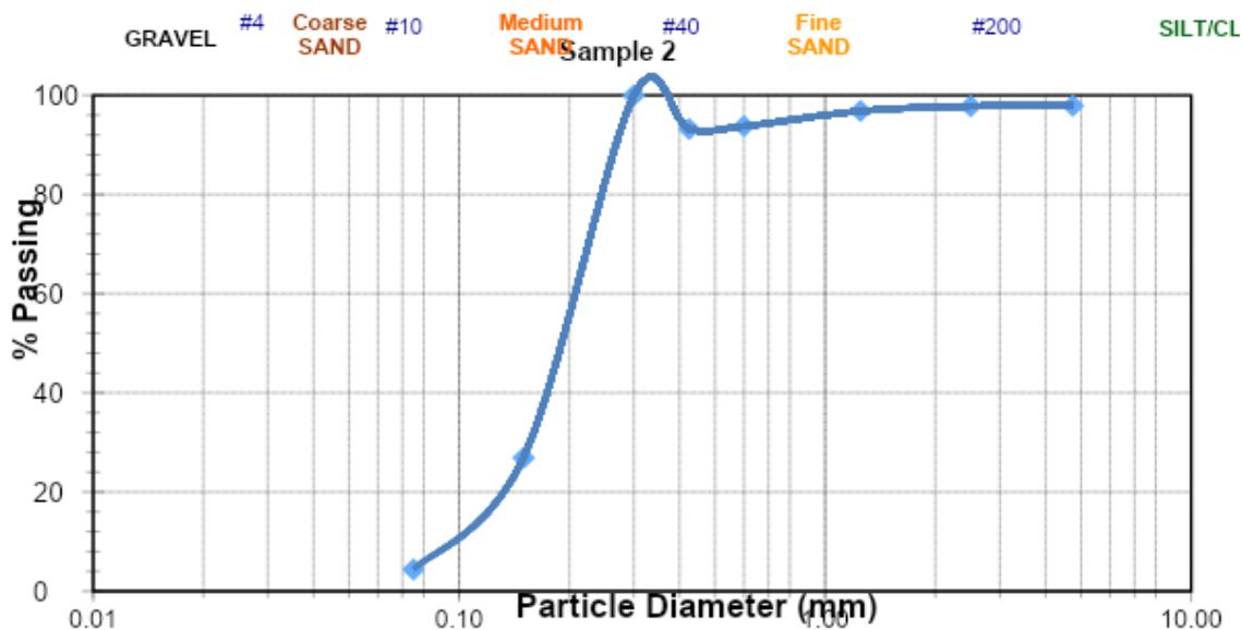
Fig. 4. Particle-size distribution of bentonite clay used in the study
